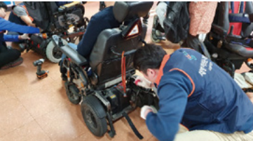
Replacement of batteries of electric wheelchairs.
